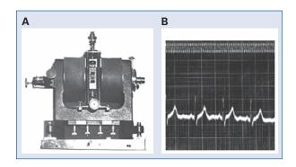
Figure 2. String galvanometer (A) and electrocardiogram recorded by it (B).
